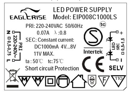
Location: attached on the enclosure and visible during installation
