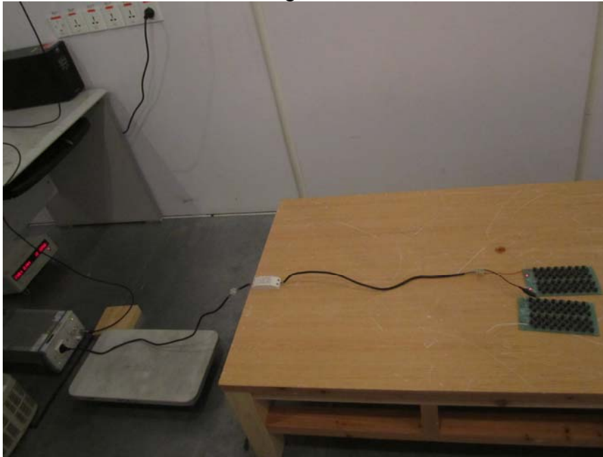
Disturbance Voltage on Mains Terminals
