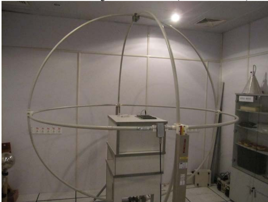
Radiated Electromagnetic Disturbance (100 kHz-30MHz)
