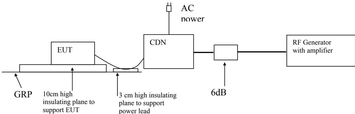
**7.2.3 Test Setup and Procedure**
