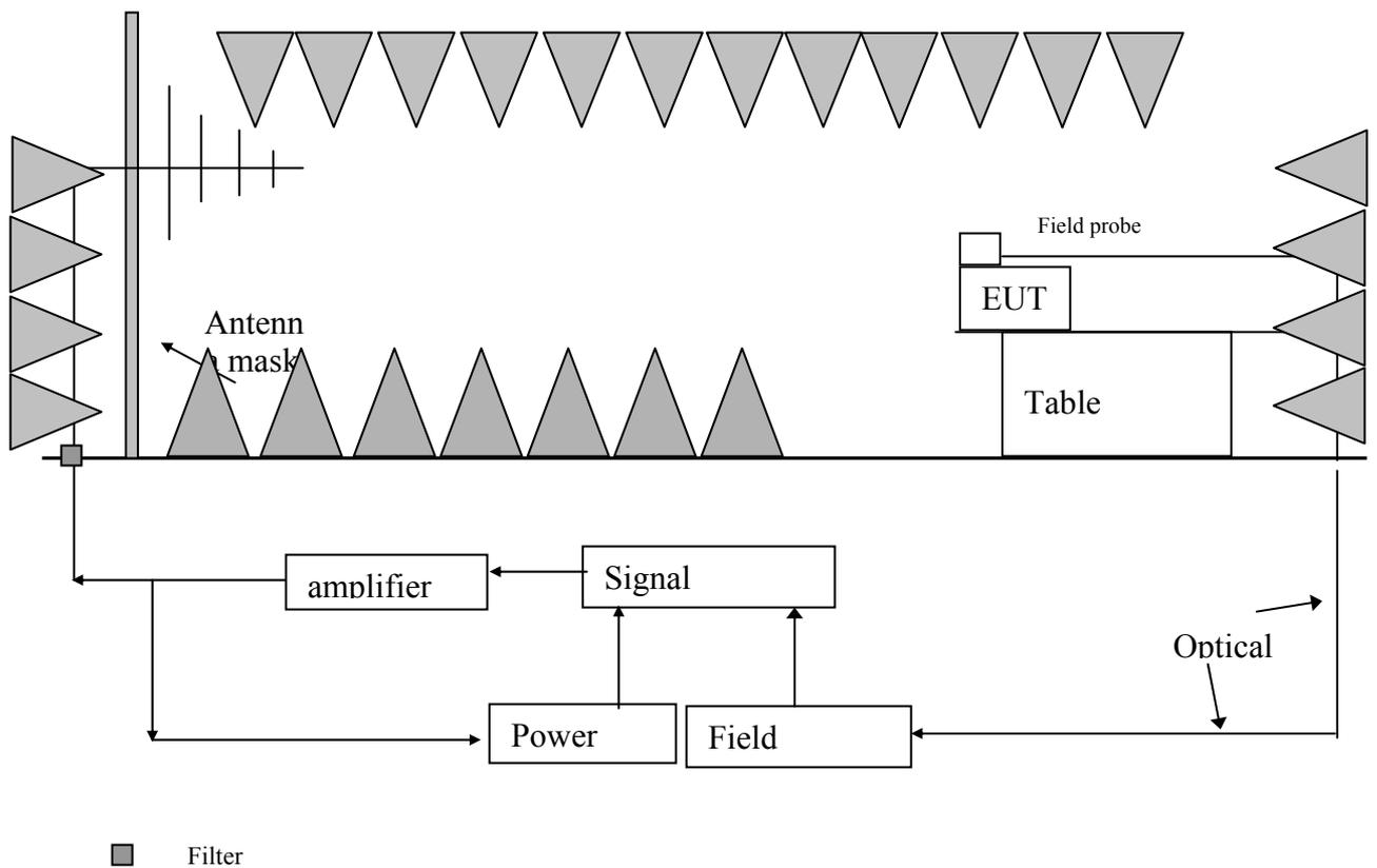
**7.6.3 Test Setup and Procedure**
