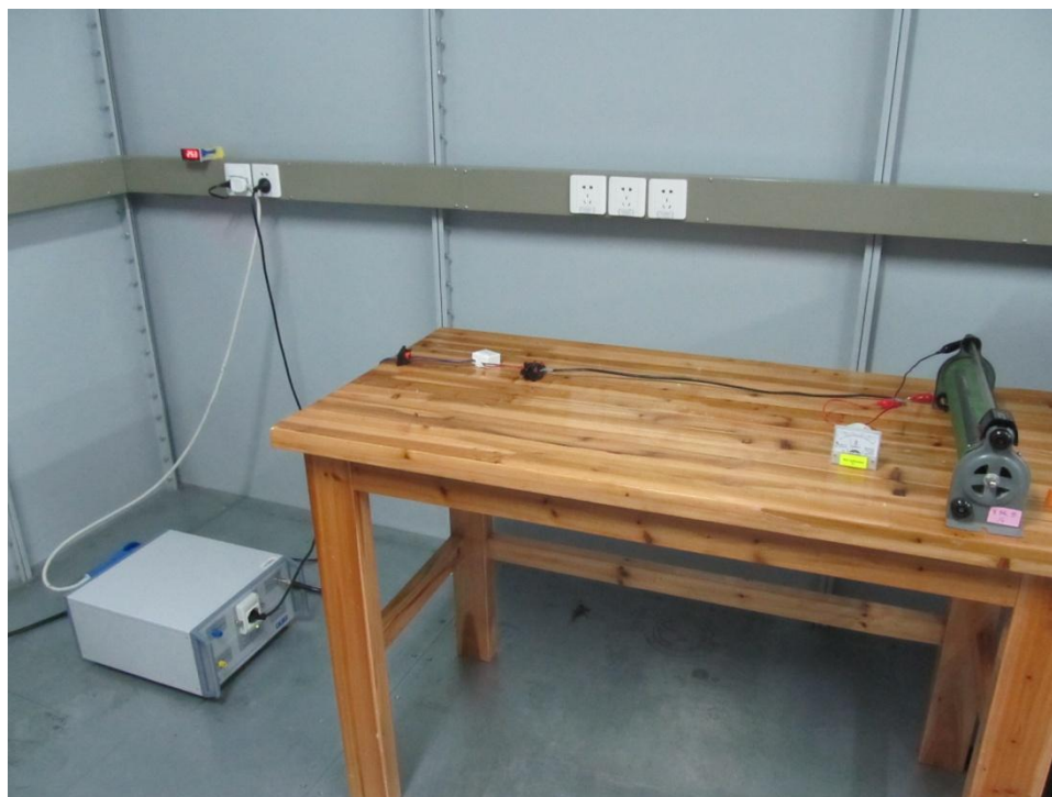
Photo of setup Conducted Emission
