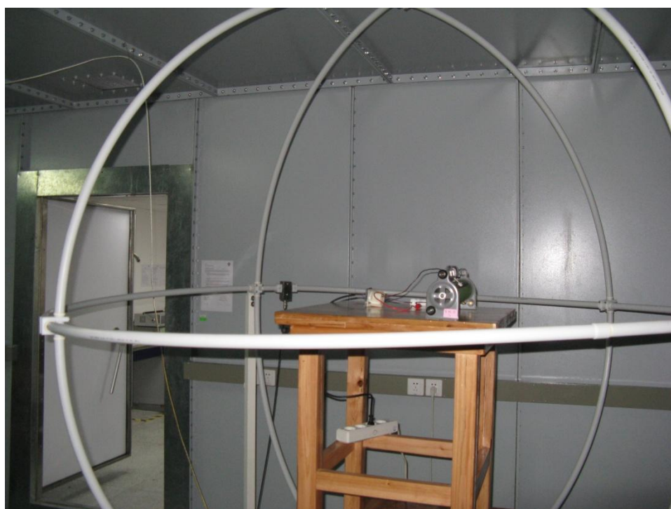
Photo of setup Radiated Emissions (Magnetic Field)
