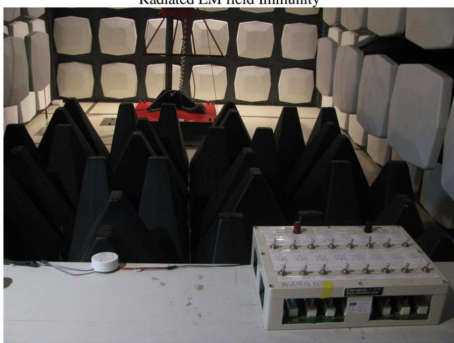
Radiated Electromagnetic Filed Disturbance (30MHz – 300MHz, CDN method)
