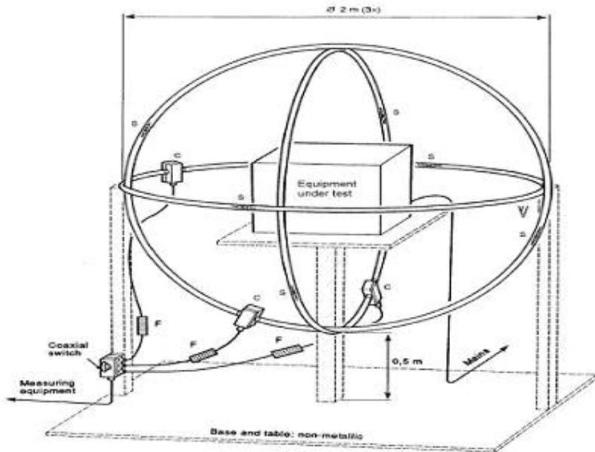
(B) Radiated Emission Test Set-Up Frequency Above 30 MHz
